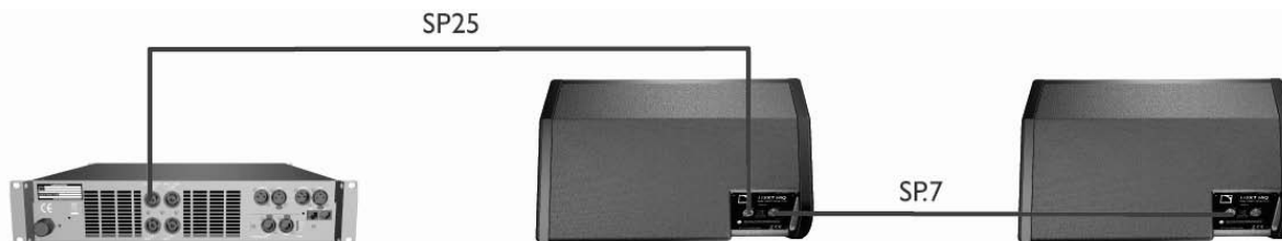
Figure 3: Connecting two 115XT HiQ in parallel to an LA4 amplified controller
