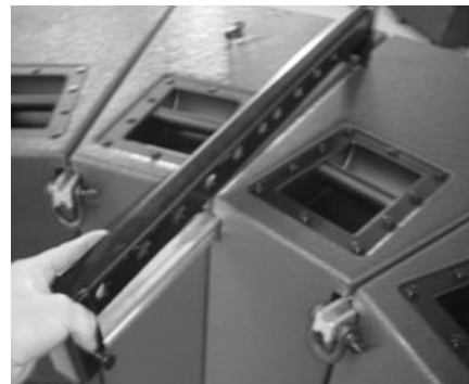
(12) BUMP3 assembly slides into position from the rear
