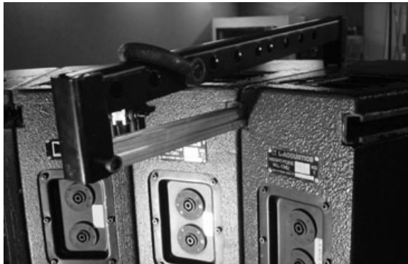
(7) BUMP3 slides into position from the rear
