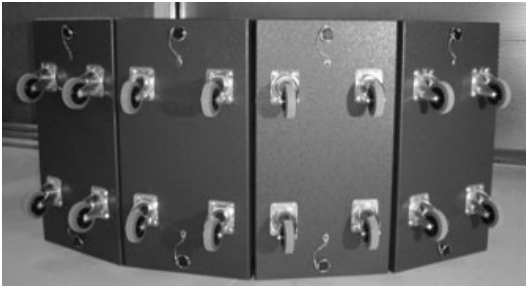
(3) Enclosures located in position and in the desired orientation (refer to rear jack plates – when facing downwards, -40 / +20 deg coverage is obtained)
