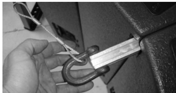
(2) Safety steels attached between ARCOUPL shackles (front and rear, top and bottom)
