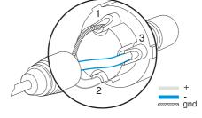
Figure 4: XLR Input Connector Wiring
