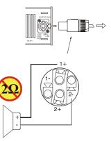
Bridged mono connection via Channel A output connector (pins I +/2-) to loudspeaker (+/-)
