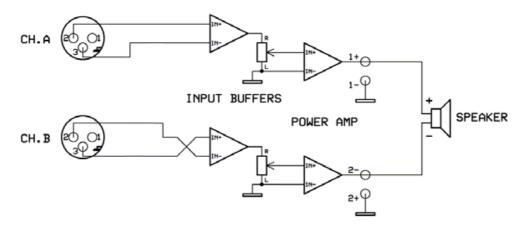
Figure 11: Reverse polarity operation for Channel B
