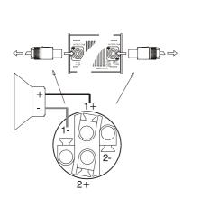
Channel A and B connected via two separate Speakons
