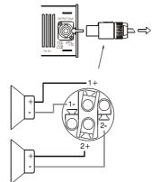
Channel A and B connected via one Speakon (for bi-amp applications)
