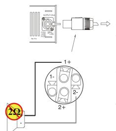
Bridged mono mode is used to deliver both channels' power to a single load. The nominal impedance of the load must be more than 4 ohms.
