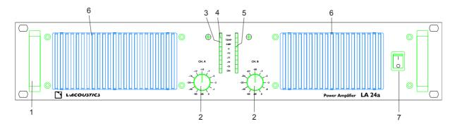
Figure I: LA24a Front Panel
