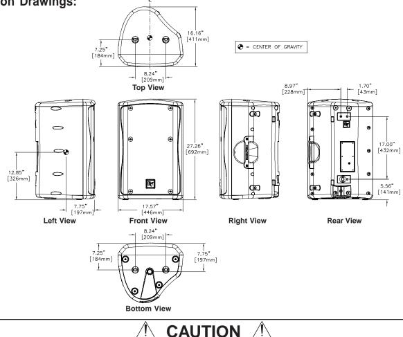
This Zx5-90PI Loudspeaker should be suspended overhead only in accordance with the procedures and limitations specified in the *Zx5 Users Manual* and possible manual update notices. This system should be suspended with certified rigging hardware by an authorized rigging professional and in compliance with local, state, and federal overhead suspension ordinances.
